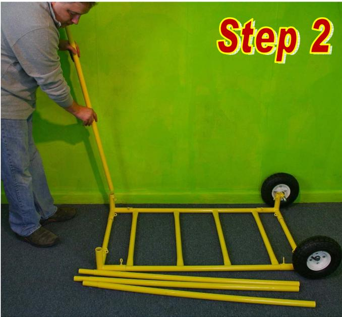
Insert a 44.5" tapered pipe in each corner fitting of the base unit. (The tapered end goes up.)
