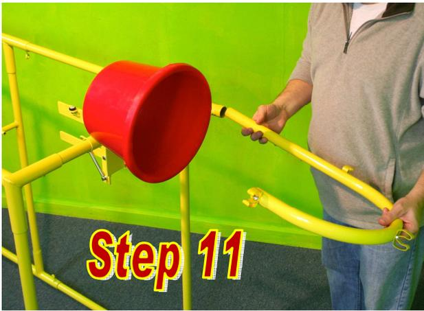
Insert filler tube hook and tighten.
